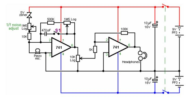
The white noise is generated by the 5-volt zener diode. The level of this white noise component is controlled by the 1.5 megohm variable resistor plus the 10K fixed limiting resistor. While the range of these two components is 10K to 1.501 Meg. the working setting is normally very high and so only a very small amount of white noise is fed into the input of the first 741 op. amp. to modify the microphone input.
